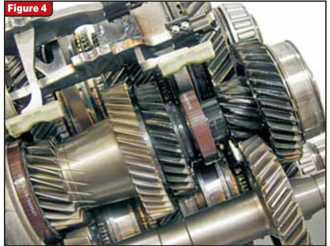
Two different colors are used to distinguish input shafts 1 and 2.
