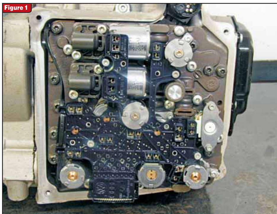
Figure 1 Valve-body and solenoid side of the Mechatronics assembly
