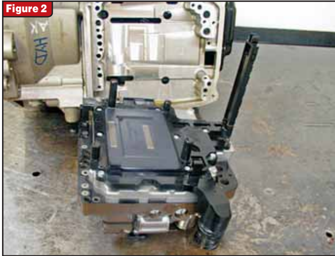
Control-module side of the Mechatronics assembly
