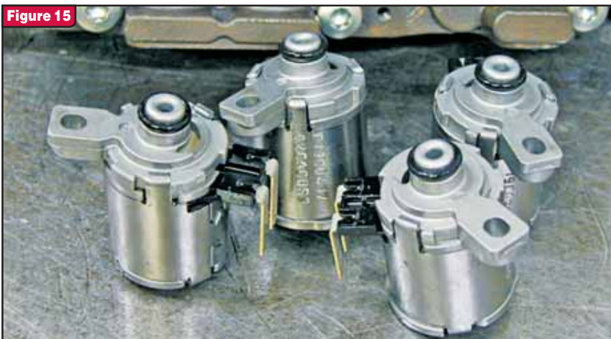
N218 pressure-control solenoid (K1/K2-clutch cooling pressure)
