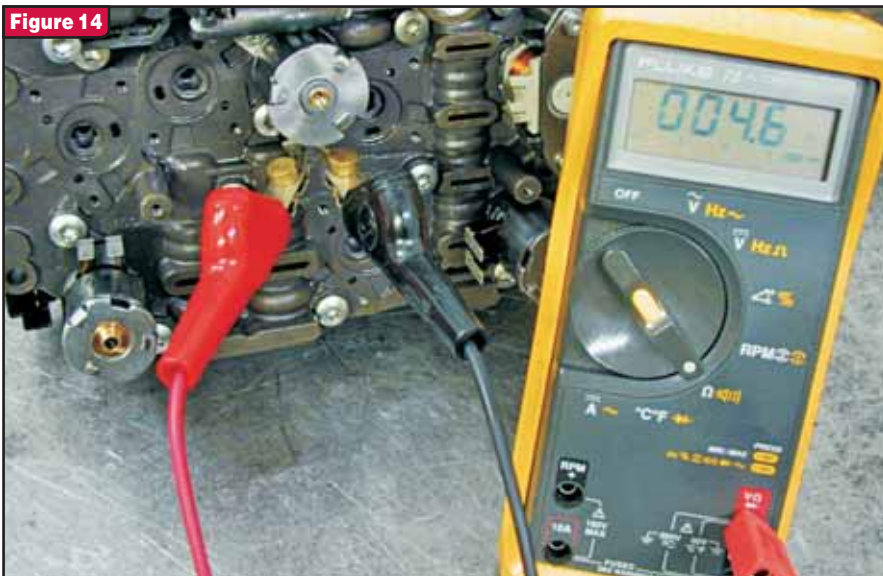
N218 pressure-control solenoid (K1/K2-clutch cooling pressure)
